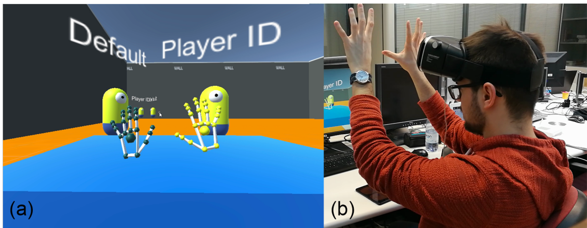
Figure 1.2: An user using the Leap Motion device mounted on a HMD to interact with the application.
