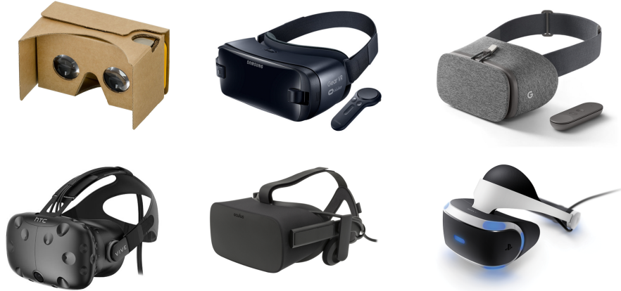
Figure 2.1: Virtual reality headsets. Starting at left from above: Google Cardboard, Samsung Gear VR, Google DayDream, HTC Vive, Oculus Rift, Playstation VR.
